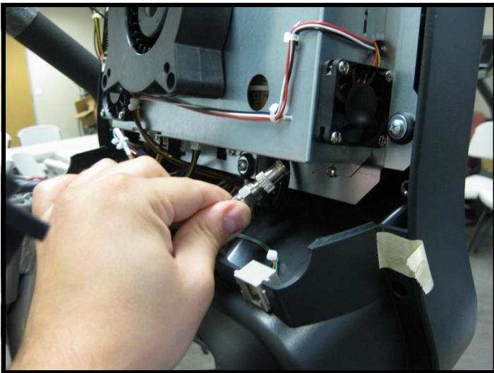
Step 15. Next plug in the coax cable to the coax adapter on the tuner card of the embedded display assembly.
